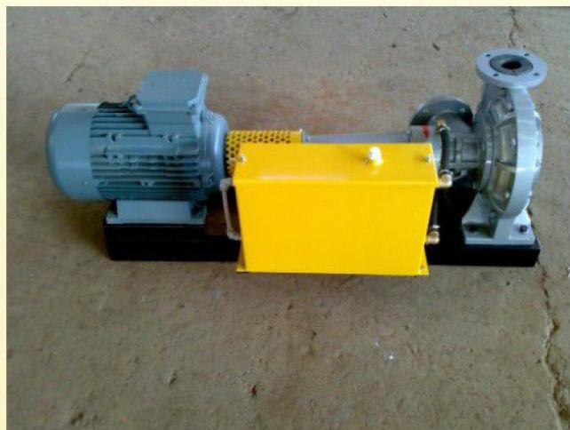
Horizontal single and two stage centrifugal type open impeller pumps.
